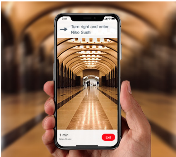
Figure 8: Image-based navigation occurs when a user takes a photo of their whereabouts in a facility and is provided with a navigation path based on their current location.
